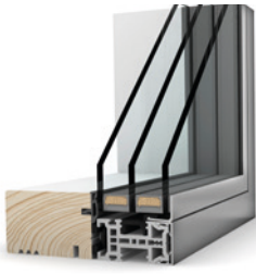
Slender window profile 42mm profile height on all fixed frame windows with 48mm glass. Perfect for large glass areas in modern buildings.
