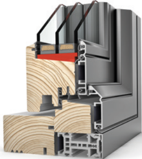
INWARD OPENING Inward opening tilt and turn windows in design style MODERN. Inward- and outward opening windows have the same frame height and can be combined in the same element.
