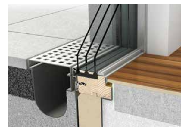
Frameless appearance and technologically optimized construction connection
